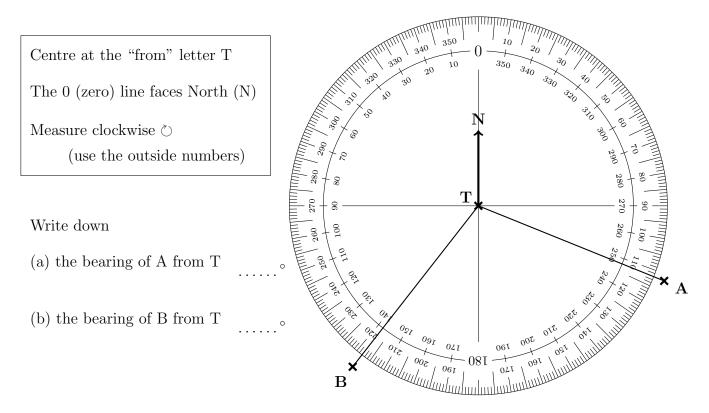
2. The diagram shows an angle measurer ready for measuring bearings from a tower T.
